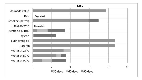
Lap shear strength versus immersion in various media (typical average values) Unless otherwise stated, L.S.S. was determined after immersion for 90 days at 23°C Cure 16 hours at 40°C
