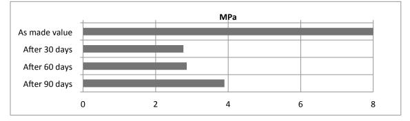
Lap shear strength versus heat ageing (typical average values)
